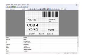
Traceability is crucial when grading and packing. When the raw material information is entered at the front of the line and is tracked and traced through production, the appropriate label can be applied on the customer package. MATRIX includes a user friendly label design program to customise labels. MATRIX allows to trace products from finished packages back to their origin of the incoming raw material.
