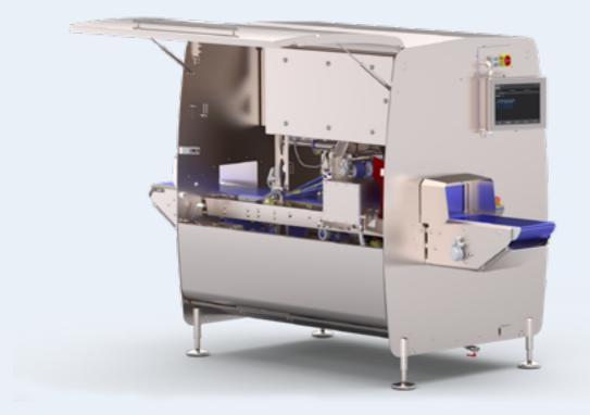
In addition to its top-mounted camera, the PORTIO Plus can be operated with two lateral cameras to create more rounded products - an effect further enhanced by a feature that can alter the angle of the knife from the 0° (vertical) position, to 30° or 45°. Cutting at an angle gives a natural look to sliced portions or creates a bigger plate coverage.
