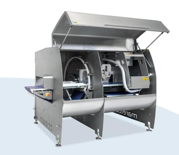
A PORTIO 3 adds two lateral cameras to the PORTIO 1. This allows the machine to improve the scanning and cover blind spots at the side of the product that cannot be detected by the top camera only. It is used for accurately portioning red meat, whole fish or any product with an irregular shape, in a vertical way. The machine can be equipped with the options mentioned on page 20.
